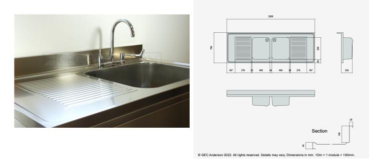
DR207 (DG45) Decimetric® 2000x700mm - double bowl, double drainer - commercial grade stainless steel sinktop. 40mm lipped front and side edges and 100x20mm rear upstand. Bowl size: 400x500x250mm deep complete with Ø38mm outlet and overflow fittings. Sound deadened and plastic protected. (EN 1.4301 grade stainless steel).
