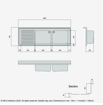
DR207 (DG65) Decimetric® 2000x700mm - double bowl, single drainer - commercial grade stainless steel sinktop. 40mm lipped front and side edges and 100x20mm rear upstand. Bowl size: 600x500x320mm deep complete with Ø38mm outlet and overflow fittings. Sound deadened and plastic protected. (EN 1.4301 grade stainless steel). LH drainer.
