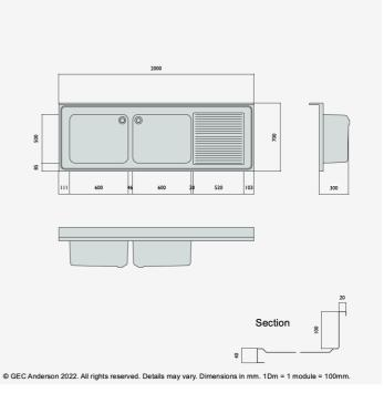
DR207 (DG65) Decimetric® 2000x700mm - double bowl, single drainer - commercial grade stainless steel sinktop. 40mm lipped front and side edges and 100x20mm rear upstand. Bowl size: 600x500x320mm deep complete with Ø38mm outlet and overflow fittings. Sound deadened and plastic protected. (EN 1.4301 grade stainless steel). RH drainer.
