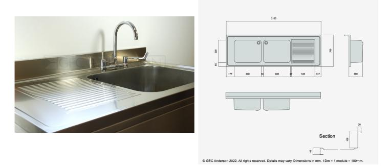
DR217 (DG65) Decimetric® 2100x700mm - double bowl, single drainer - commercial grade stainless steel sinktop. 40mm lipped front and side edges and 100x20mm rear upstand. Bowl size: 600x500x320mm deep complete with Ø38mm outlet and overflow fittings. Sound deadened and plastic protected. (EN 1.4301 grade stainless steel). RH drainer.
