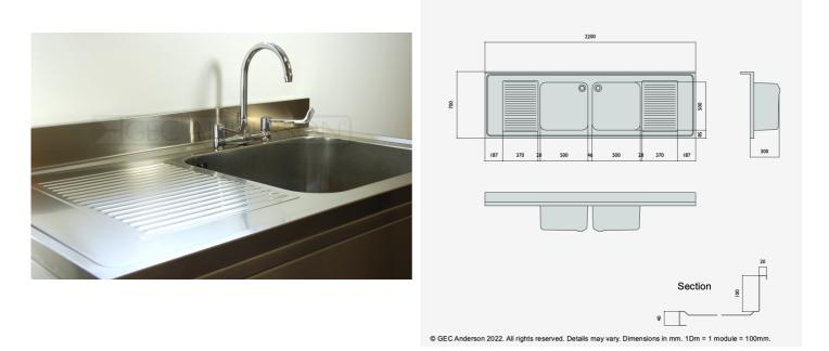
DR227 (DG55) Decimetric® 2200x700mm - double bowl, double drainer - commercial grade stainless steel sinktop. 40mm lipped front and side edges and 100x20mm rear upstand. Bowl size: 500x500x300mm deep complete with Ø38mm outlet and overflow fittings. Sound deadened and plastic protected. (EN 1.4301 grade stainless steel).
