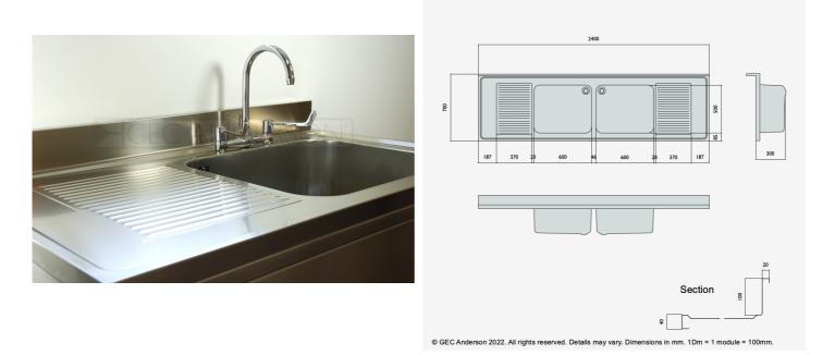
DR247 (DG65) Decimetric® 2400x700mm - double bowl, double drainer - commercial grade stainless steel sinktop. 40mm lipped front and side edges and 100x20mm rear upstand. Bowl size: 600x500x300mm deep complete with Ø38mm outlet and overflow fittings. Sound deadened and plastic protected. (EN 1.4301 grade stainless steel).
