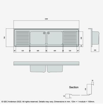
DR257 (DG65) Decimetric® 2500x700mm - double bowl, double drainer - commercial grade stainless steel sinktop. 40mm lipped front and side edges and 100x20mm rear upstand. Bowl size: 600x500x320mm deep complete with Ø38mm outlet and overflow fittings. Sound deadened and plastic protected. (EN 1.4301 grade stainless steel).
