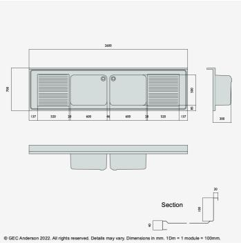
DR267 (DG65) Decimetric® 2600x700mm - double bowl, double drainer - commercial grade stainless steel sinktop. 40mm lipped front and side edges and 100x20mm rear upstand. Bowl size: 600x500x320mm deep complete with Ø38mm outlet and overflow fittings. Sound deadened and plastic protected. (EN 1.4301 grade stainless steel).
