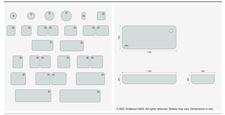
G125 single bowl: 1160x500x200mm. Complete with Ø38mm waste and overflow fittings.
