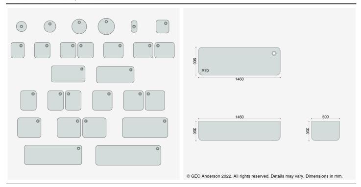
G155 single bowl: 1460x500x350mm. Complete with Ø38mm waste and overflow fittings.
