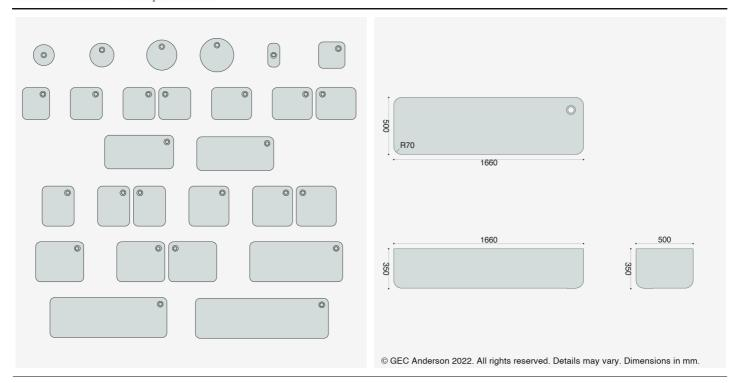
G175 single bowl: 1660x500x350mm. Complete with Ø38mm waste and overflow fittings.
