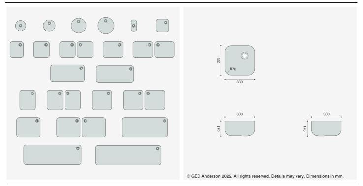
G33 single bowl: 330x330x170mm. Complete with Ø38mm waste and overflow fittings.
