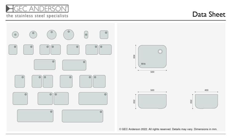
G54 single bowl: 500x400x250mm. Complete with Ø38mm waste and overflow fittings.
