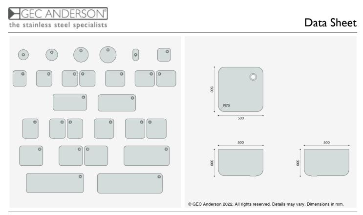
G55 single bowl: 500x500x300mm. Complete with Ø38mm waste and overflow fittings.
