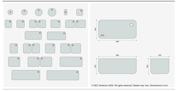
G94 single bowl: 860x420x350mm. Complete with Ø38mm waste and overflow fittings.
